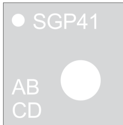
Figure 16 Top view of the SGP41 illustrating the laser marking.
