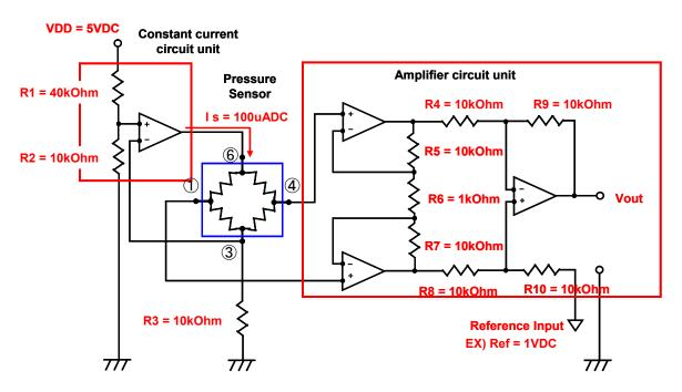
Fig. 7 Example of Recommended Circuit Diagram for 2SMPP-02
