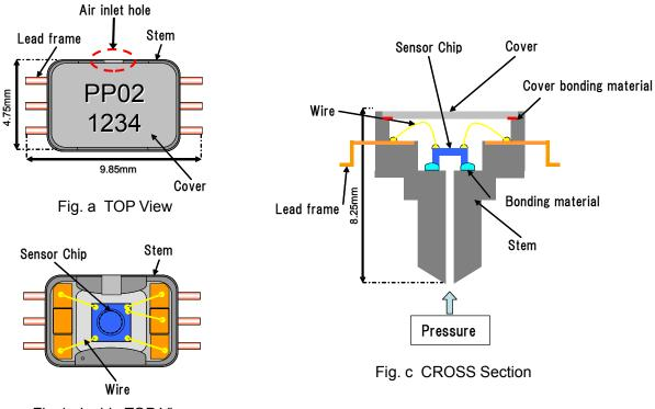
Fig. b Inside TOP View
