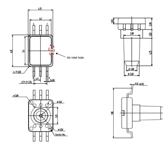
The recommended tube inside diameter is 2 mm.
