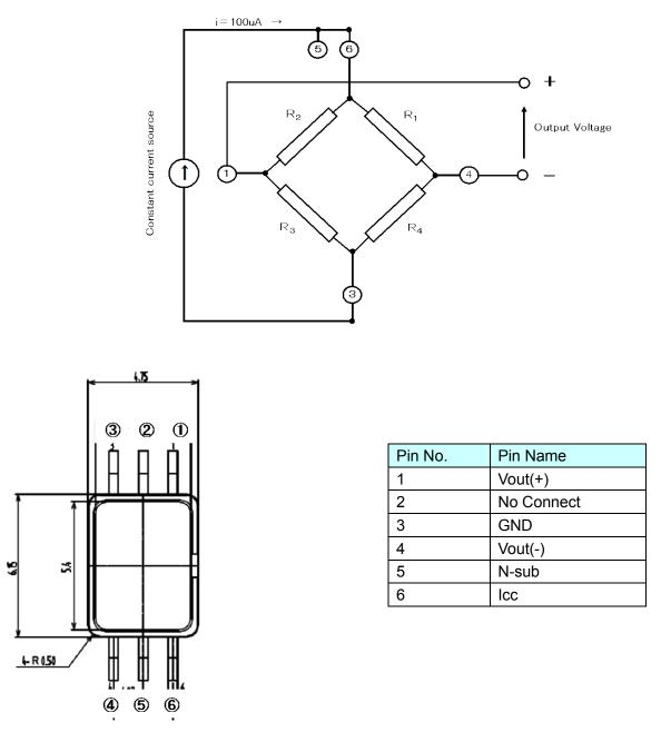
Fig.5 Equivalent Circuit and Connection Diagram of 2SMPP-02
