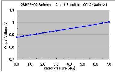
Fig.9 Output characteristic of 2SMPP-02 after Gain=21 times
