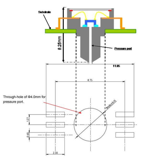
Fig. 6 Recommended Mounting PAD Layout of 2SMPP-02
