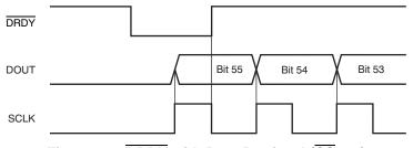
Figure 30.  $\overrightarrow{DRDY}$  with Data Retrieval ( $\overrightarrow{CS} = 0$ )
