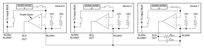
Figure 48. RLD Connection for Multiple Devices
