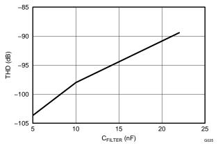
Figure 19. THD versus C<sub>FILTER</sub> Value
