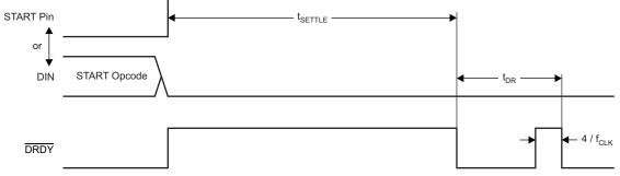
(1) Settling time uncertainty is one  $t_{\mbox{MOD}}$  cycle.
