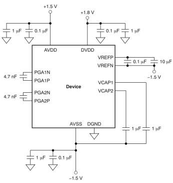
NOTE: Place the capacitors for supply, reference, VCAP1, and VCAP2 as close to the package as possible.
