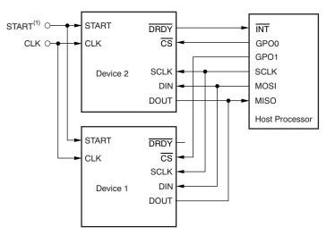
Figure 37. Multiple Device Configurations
