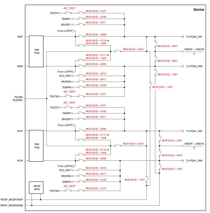
NOTE: MVDD monitor voltage supply depends on channel number; see the Supply Measurements (MVDDP, MVDDN) section.
