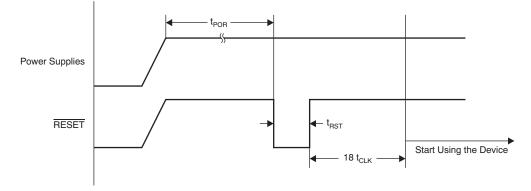
Figure 51. Power-Up Timing Diagram
