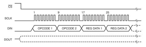
Figure 41. WREG Command Example: Write Two Registers Starting from 00h (ID Register) (OPCODE 1 = 0100 0000, OPCODE 2 = 0000 0001)
