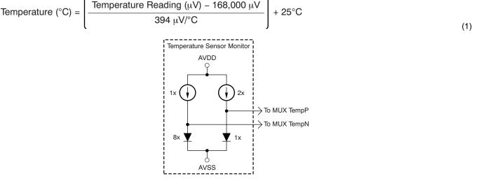
Figure 15. Measurement of the Temperature Sensor in the Input
