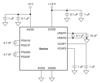
NOTE: Place the capacitors for supply, reference, VCAP1, and VCAP2 as close to the package as possible.
