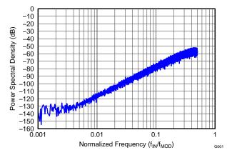
Figure 20. Power Spectral Density (PSD) of a ΔΣ Modulator (4-Bit Quantizer)
