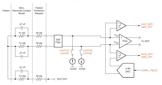
NOTE: The R<sub>P</sub> value must be selected in order to be below the maximum allowable current flow into a patient (in accordance with the relevant specification the latest revision of IEC 60601).
