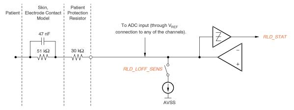
NOTE: The R<sub>P</sub> value must be selected in order to be below the maximum allowable current flow into a patient (in accordance with the relevant specification the latest revision of IEC 60601).
