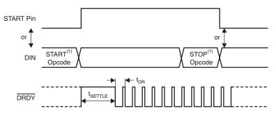
(1) START and STOP opcode commands take effect on the seventh SCLK falling edge at the end of the opcode transmission.
