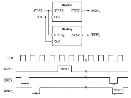
(1) Start pulse must be at least one  $t_{\mbox{MOD}}$  cycle wide.
