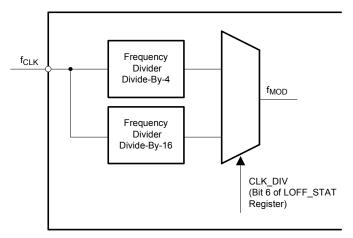
Figure 28. Relationship Between External Clock (f<sub>CLK</sub>) and Modulator Clock (f<sub>MOD</sub>)
